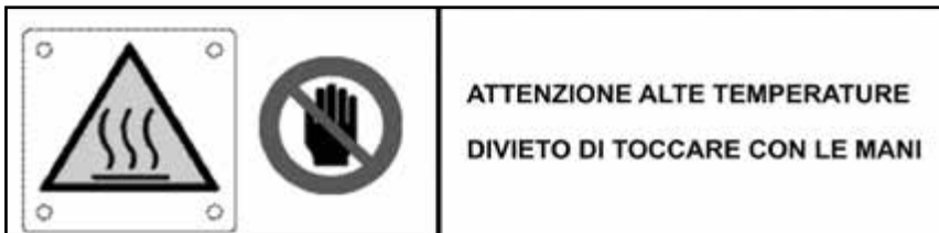
Fig. 2 - Security labels installed on the oven
